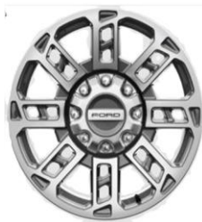
20" Bright Machined and Carbonized Gray High-Gloss Painted Aluminum; Gloss Black Hub Cover/Center Ornament (Incl. w/ Platinum Plus Package) – 64L
